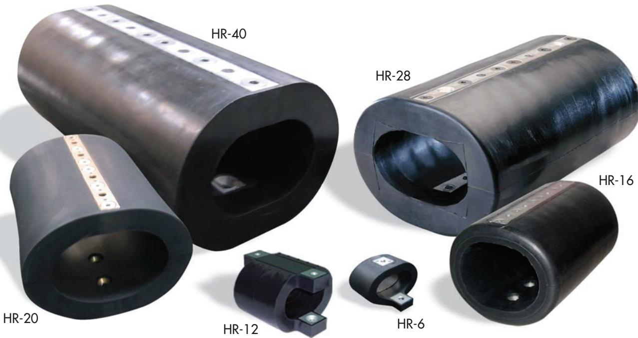
The HERM isolator incorporates the use of a traditional Enidine helical wire rope isolator encased in a proprietary elastomeric compound. The stainless steel cable of the mount provides for a rugged construction, while the elastomer provides additional damping and stiffness. This unique design results in a fail safe mount with a higher stiffness and energy absorption capacity.
